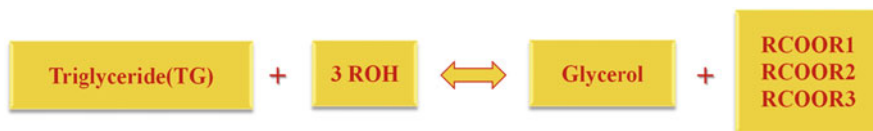
Fig. 10.2 Transesterification reaction resulting in the production of biodiesel and glycerol. Adapted from Caetano et al. (2018)
