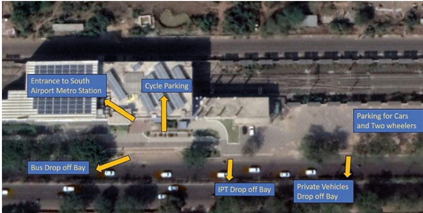
Fig. 2 Schematic representation of arrangements for different modes near the South Metro station area
