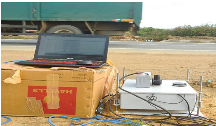
Fig. 4 Field snapshot of IR sensor device set up across the highway segment
