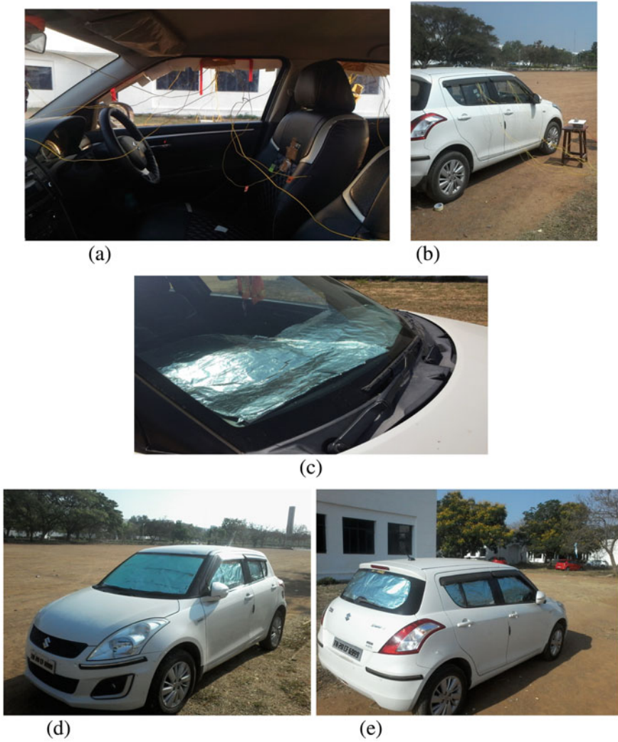
Fig. 2 Pictorial view of the experimental setup a thermocouple locations within the cabin, b outside view of the car during Case-1 experiments, c view of the radiation shield on the dashboard (Case-3), d and e respective front and rear views of the radiation shielded car prepared for Case-4 studies
