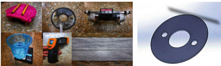
Fig. 2 All materials used for electrically driven interfacial evaporation setup and the corresponding disc heater CAD model
