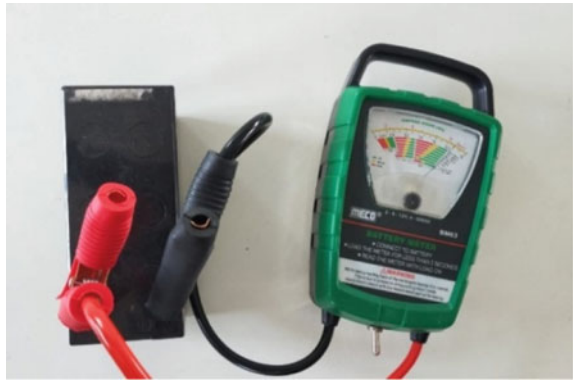
Fig. 16 Li-ion battery with battery meter
