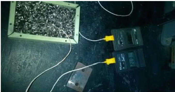
Fig. 3 Arrangement of the thermocouple inside the aluminum shots and the connection to the temperature display
