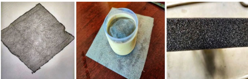
Fig. 1 Materials used for solar-based interfacial evaporation setup: spunlace fabric, insulated beaker, ester-based polyurethane foam
