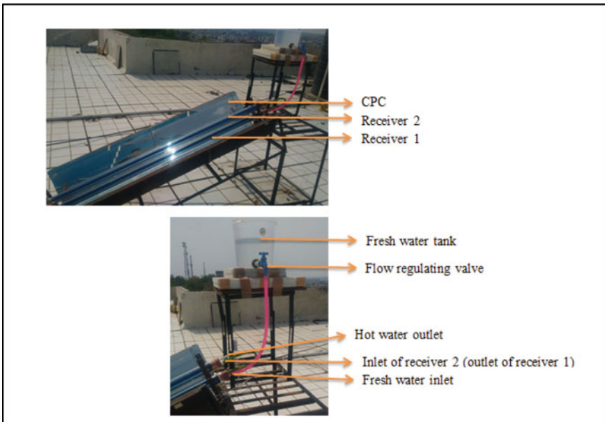
Fig. 9 Experimental setup of fresh water inlet condition using two receivers
