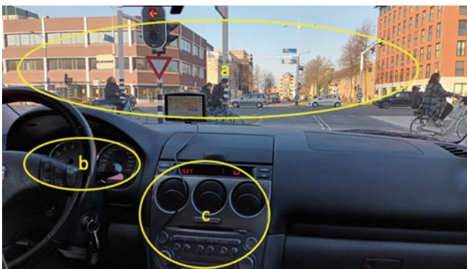
Fig. 9.7 Areas available for distribution of UI functions. a Primary line of sight; b Dash panel; c Mid panel/console
