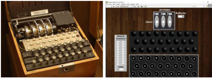
Fig. 7.10 The left side shows the original ENIGMA Machine. On the right is the digital version of the ENIGMA Machine implemented in LabVIEW
