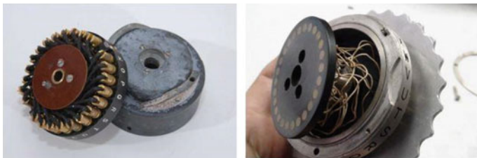
Fig. 7.7 The reflector’s internal wiring is shown on the left; a rotor’s internal wiring is shown on the right
