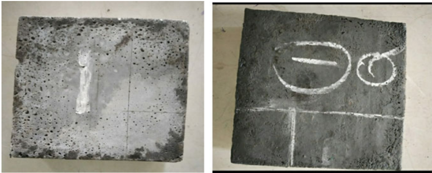
Fig. 5 Paver block after removing from mould
