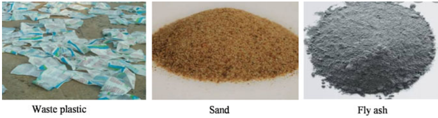
Fig. 2 Material used for preparing paving block
