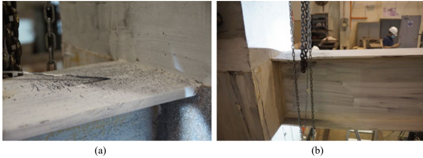
Fig. 8 Images of the specimen showing a flange yielding and b flange local buckling at the beam plastic hinge region
