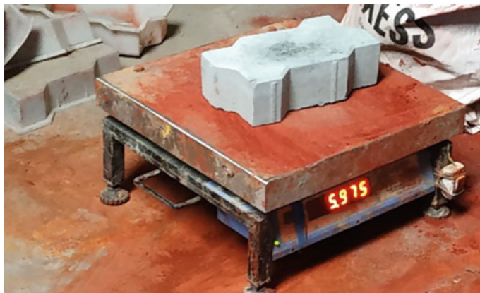
Fig. 4 Measuring the mass of tested sample having surface area of 0.0322578 \text{ m}^2 with a height of 80 mm
