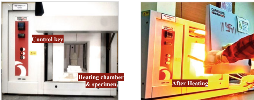
Fig. 5 Exposure of CALS mortar mix at temperature of 800 °C ± 5 °C in a high-temperature furnace (Make: M/s. CarboliteGero, GmbH)
