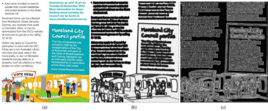
Fig. 2.5 Spatial adaptive divisive normalized parameters visualization for classical SCI (darker pixels denote higher normalization parameters). a Pristine SCI; b Normalization parameters obtained from SSIM; c Normalization parameters accessed from SSI ([©2021] IEEE. Reprinted, with permission, from [29].)
