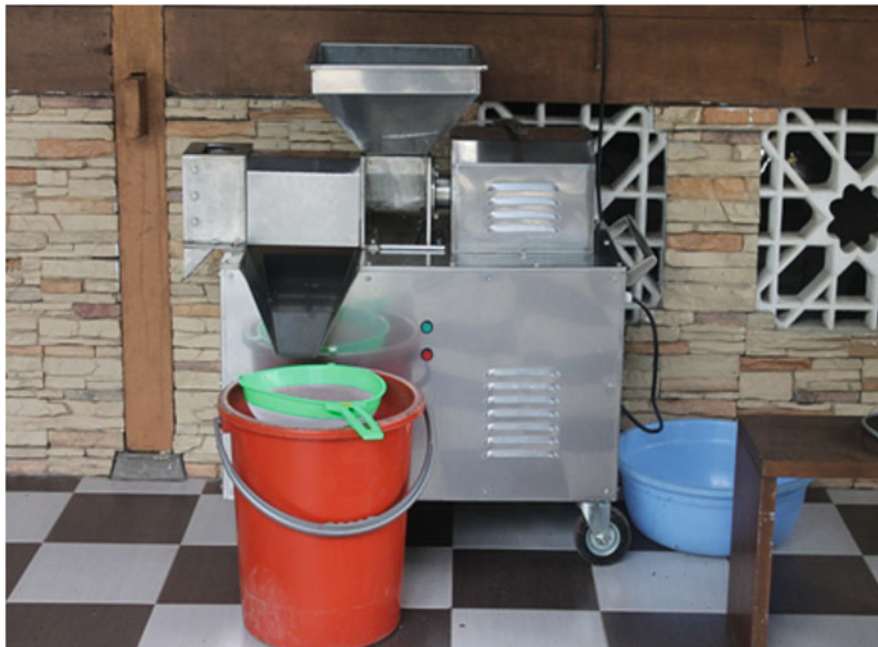
Fig. 10.14 Sugar palm sago extruder machine for extracting starch
