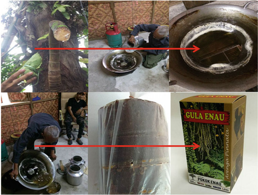
Fig. 10.16 The production of sugar palm block starting from sap collection until packaging
