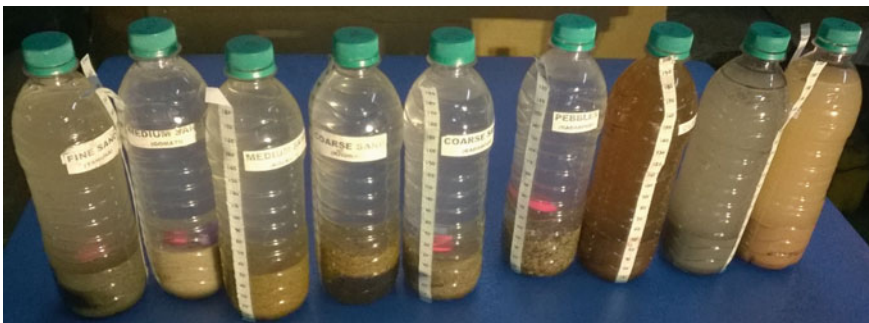
Fig. 5 Nine Soil specimens in 500 ml bottle subjected to finger tapping as external excitation
