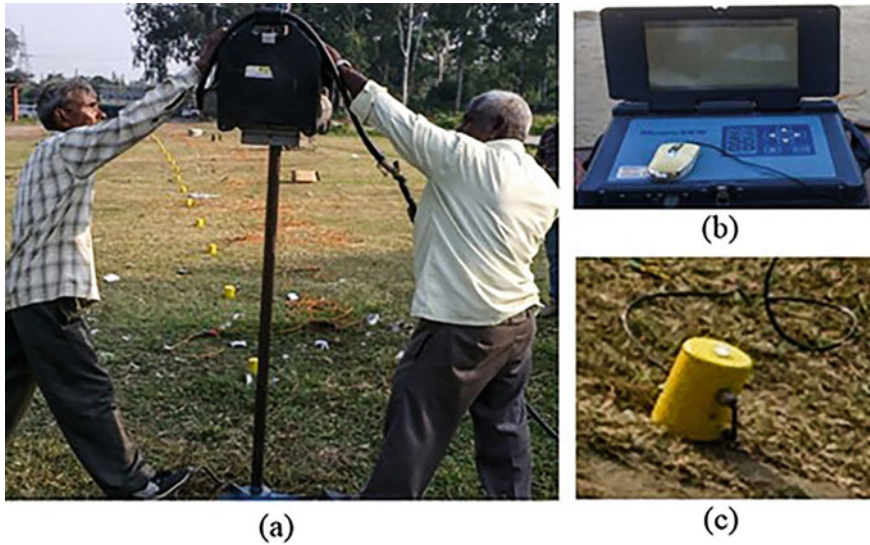
Fig. 7 MASW test setup: a Drop weight arrangement and receiver array, b A sample recording device: McSeis-SXW 24 channel seismograph, and c A sample vertical component geophone (Roy & Jakka, 2018)
