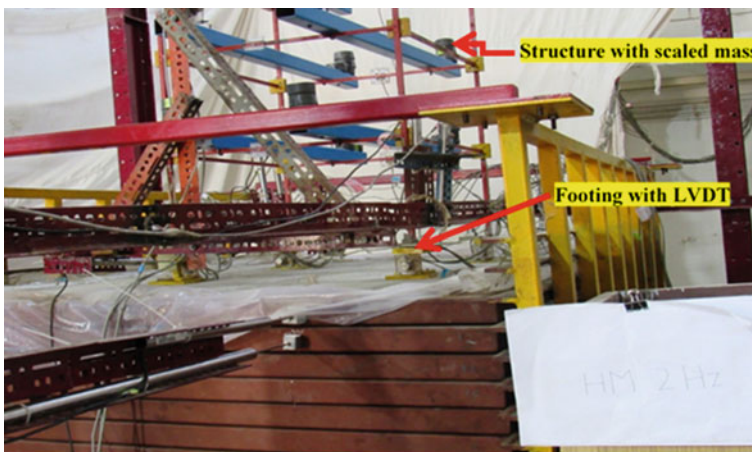
Fig. 3 Photograph of the instrumented structure–foundation system on laminar soil box
