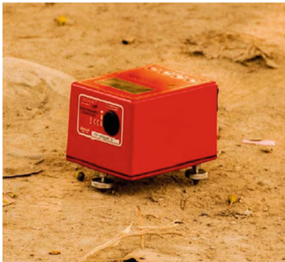
Fig. 12 A single station 3-component ambient vibration recording sensor to obtain H/V spectral ratio curve
