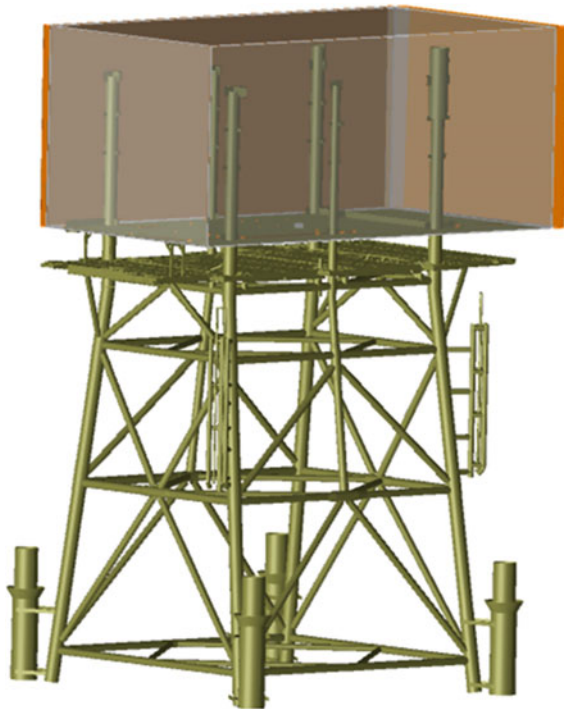
Fig. 17 Analysis of offshore substation structure
