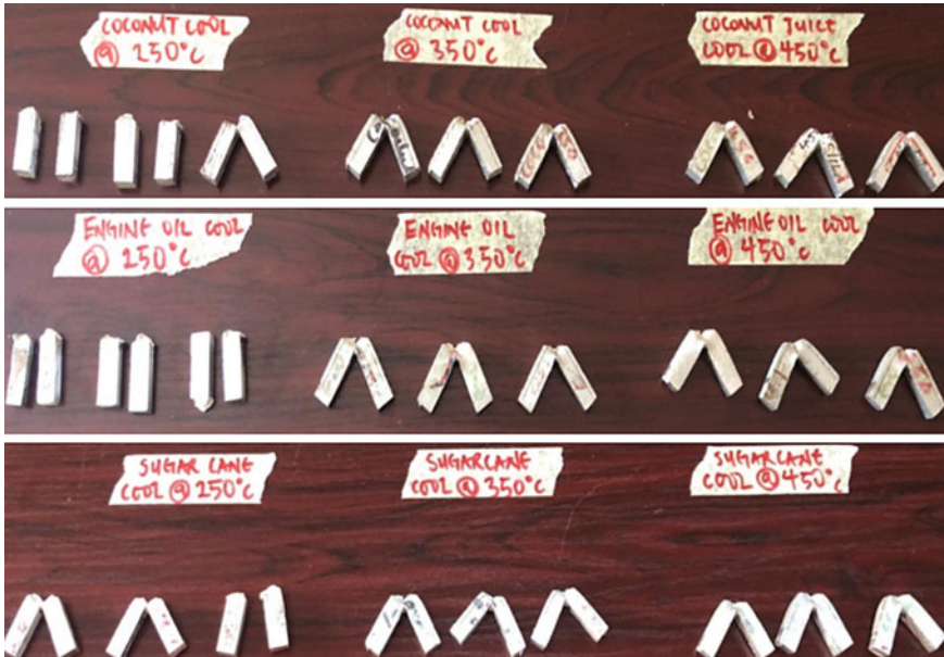
Fig. 1 Images of fractured specimen after carrying out impact test
