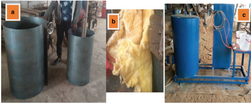
Fig. 3 a Outer and inner layers of the combustion chamber. b Lagging with fibre glass. c Fabricated and assembled gasifier system
