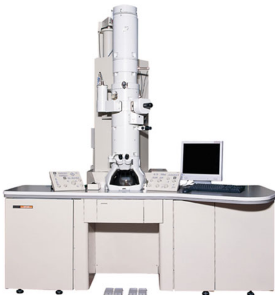
Fig. 5.3 Experimental set-up for transmission electron microscopy (JEOL JEM2010)
