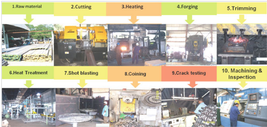
Fig. 3 Manufacturing process of forged steel crankshaft [9, 11] Source Forge & Forge Pvt. Ltd. Rajkot
