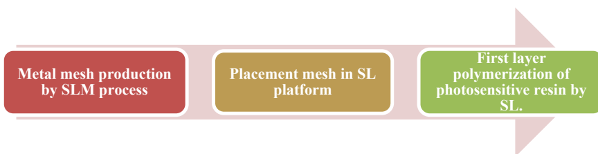
Fig. 8 Stages of sample preparation
