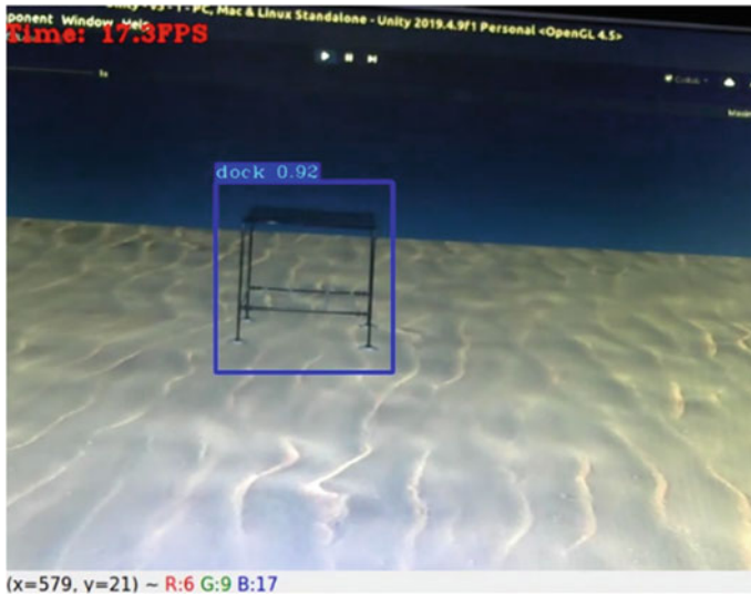
Fig. 5 Screenshot of the algorithm detecting the dock in simulation
