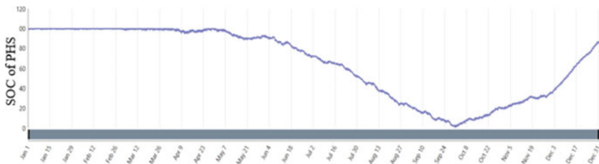
Fig. 7 State of charge of PHS for PV-WT-PHS configuration
