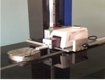
Fig. 2. Measurement of Ra.
