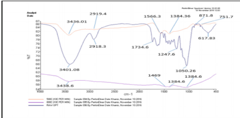
Fig. 2. The FTIR spectra of raw oil palm trunk powder and oil palm trunk powder that passed heat treatment at temperature 500 °C and 800 °C for 10 °C/min heating rate and 2-h soaking time.
