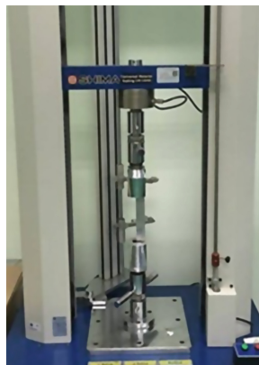
Fig. 3. The strengths of the single lap joints were determined from tensile testing machine.
