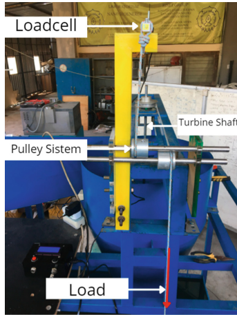
Fig. 1. Prony brake system schematic.
