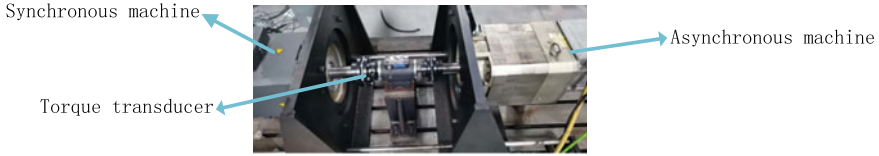
Fig. 10 Experiment platform for stray flux measurement
