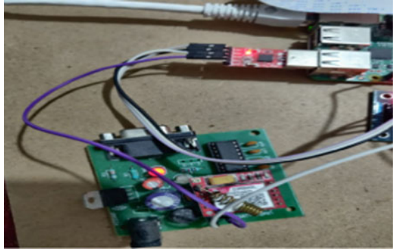
Fig. 2.6 GSM module interfacing with Raspberry PI
