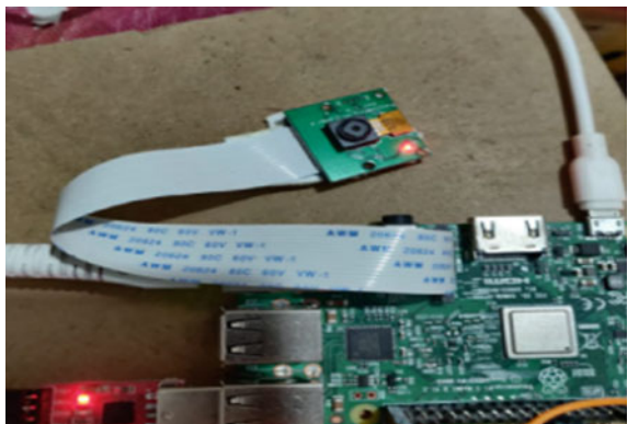
Fig. 2.5 Camera connected for face recognition
