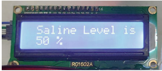
Fig. 12 Output on the LCD screen for saline level
