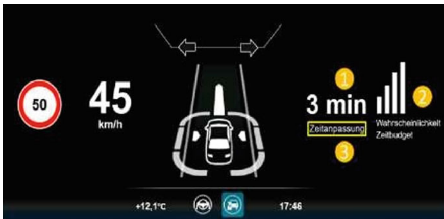
Fig. 3 Design of a HMI that notifies the operator of the rationale for an urgent maneuver’s activation
