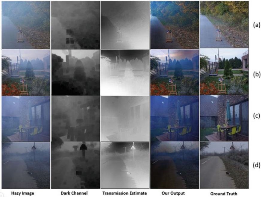
Fig. 6 First hazy image from OHAZY dataset. Then its dark channel after that the scene radiance then at fourth the output after dark channel prior and at the end ground truth
