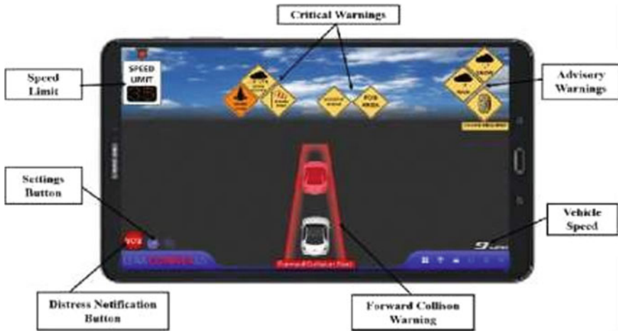
Fig. 2 Depicts an HMI notifying the motorist of the system-selected action (CF manoeuvre in this case)
