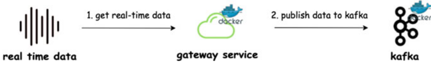
Fig. 6 Gateway service architecture. Gateway service is used as the entry point to the Rahasak-ML platform. It fetches (or pushes from other services) real-time data from various data sources such as log fields, NetFlow, TCP, UDP, and database
