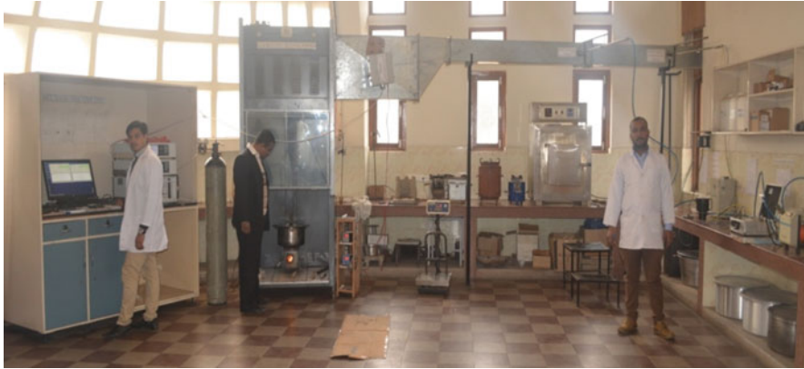
Fig. 9.1 Cookstove test center showing different measuring equipment with cookstove testing hood
