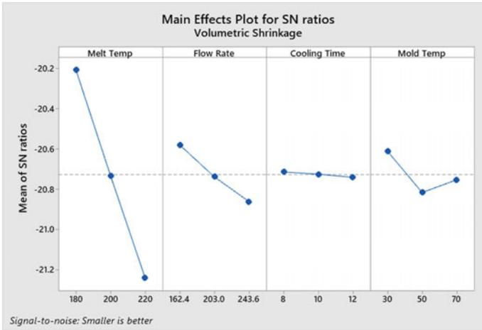
Fig. 2 Main effects plot for S/N ratios of volumetric shrinkage
