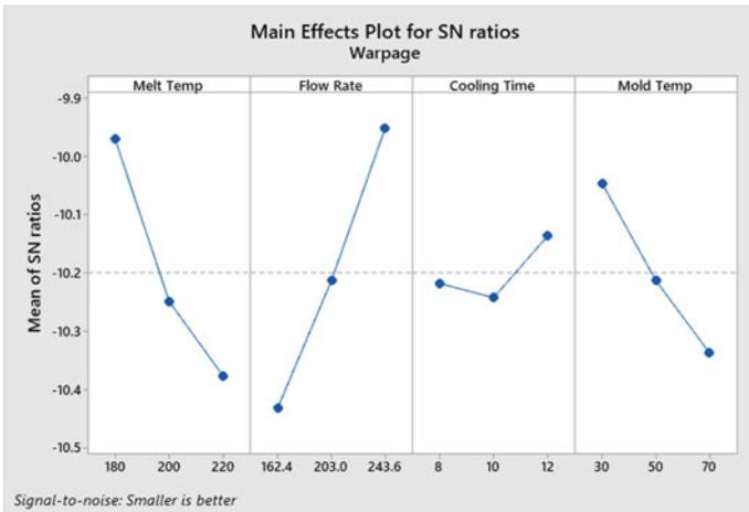
Fig. 3 Main effects plot for S/N ratios of warpage
