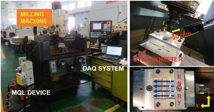
Fig. 2 Machining setup, nozzle distance and cutting path
