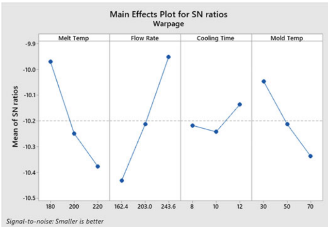
Fig. 3 Main effects plot for S/N ratios of warpage
