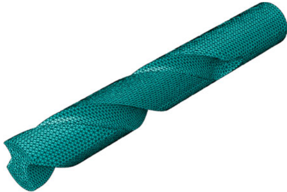
Fig. 3 Tetrahedral meshing of cutting tool
