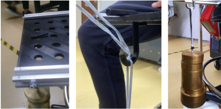
Fig. 10 Pegboard position during the test (left), installation of hanging hook onto the pegboard from the bottom (middle), load testing applied on the hanging hook (right)
