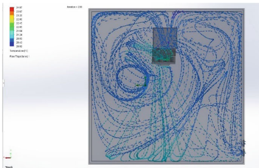
Fig. 4 First case of the CFD simulation without heat sink
