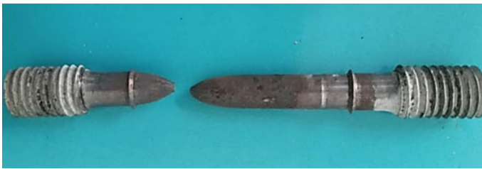
Fig. 3 Fractured specimen of P91 steel
