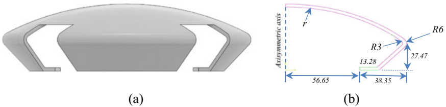
Fig. 3 a Body cover and b axisymmetric section of the body cover with thickness 3 mm
