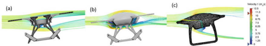
Fig. 9 Streamlines around a original RFS drone b modified RFS drone c DJI Phantom 4
