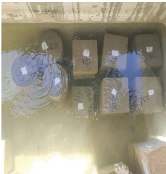
Fig. 4 Specimens placed at water basin for curing
