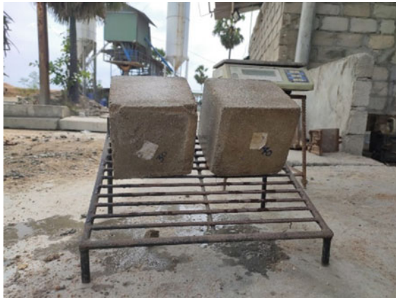
Fig. 8 Keep the cubes to rest for drying surface water
