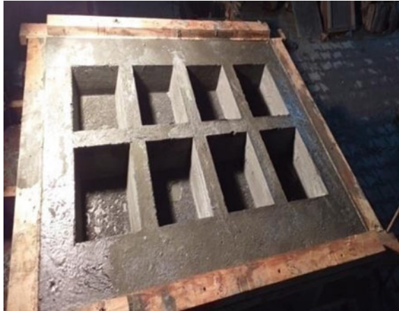
Fig. 20 UHPC waffle deck panel
