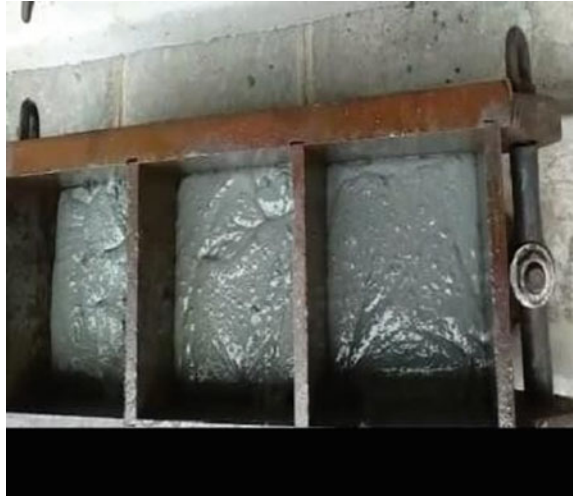
Fig. 5 Casting UHPC cubes
