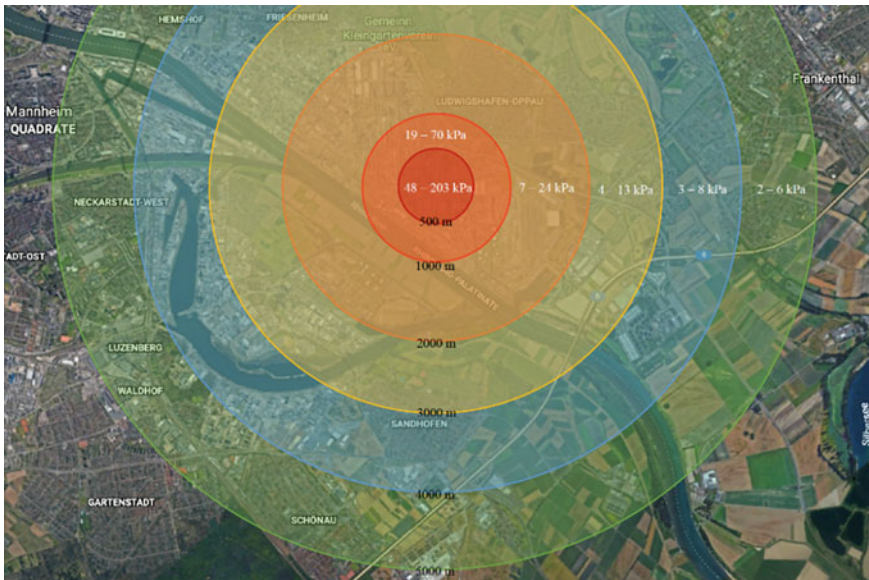
Fig. 6 Heat map for the Oppau explosion for a range of 0.7–2.8 kt TNT
