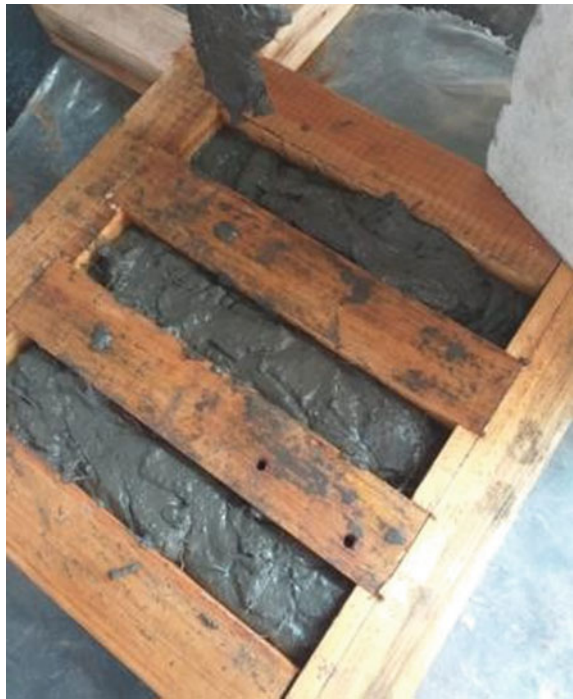
Fig. 7 Casting of the prisms
