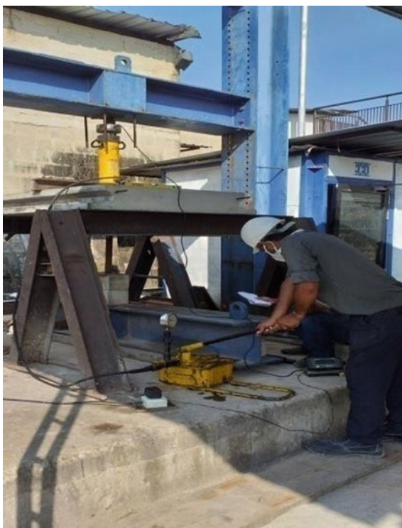
Fig. 22 Concentration load test of panel
