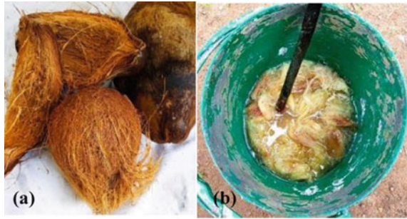
Fig. 1 a Raw coir fibre with coconut husk, b coir fibres during alkaline hydrogen peroxide pre-treatment
