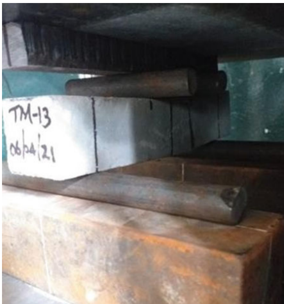
Fig. 8 Flexural strength test of UHPC
