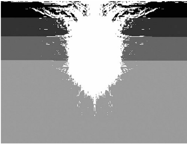
Fig. 50 Destruction of explosion at a depth of 1.25 m
