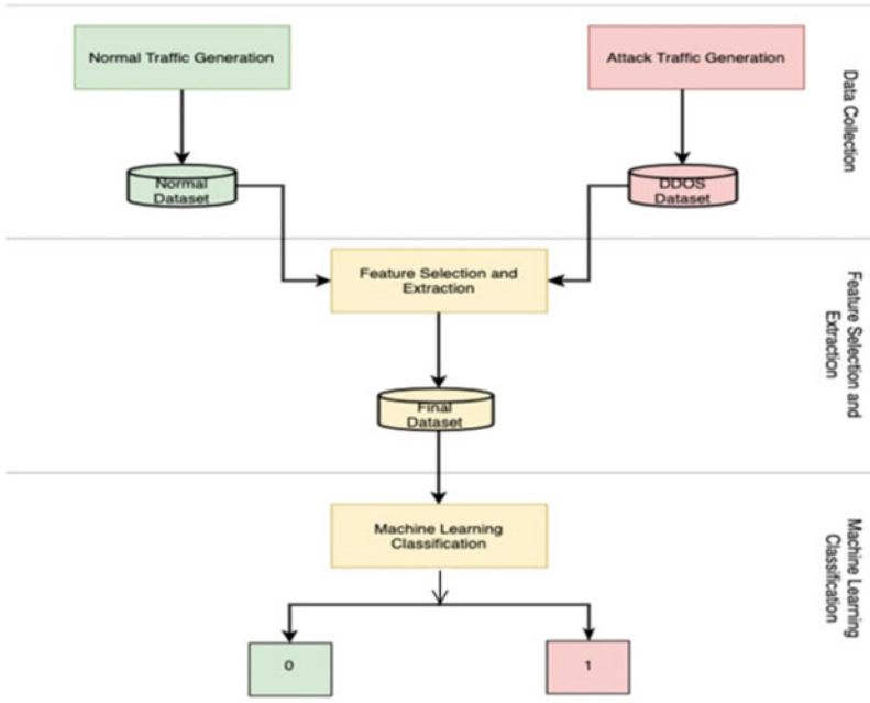
Fig. 6 Procedure for the developed testbed
