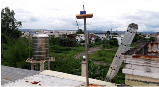
Fig. 5 The gateway on top of a building in order to have LOS conditions
