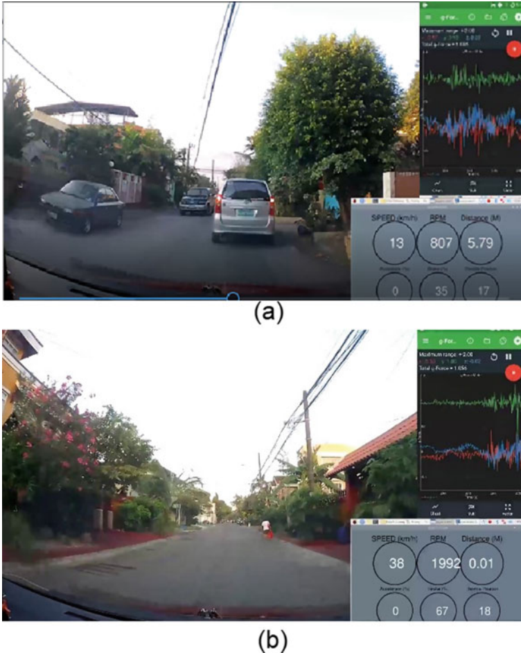
Fig. 6 Readings when the test vehicle detects an obstacle in (a) and an empty space in (b). We note that incoming vehicles are not detected by system if it is found in the other lane. Also, the bicycle is not also detected by the system
