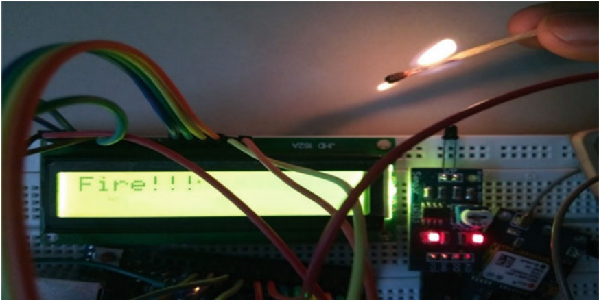
Fig. 3 Output on LCD when fire sensor detects fire nearby
