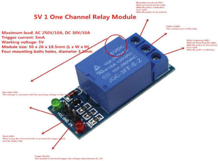
Fig. 5 Relay pin diagram
