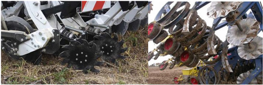
Fig. 24.7 Some types of direct sowing machines used in sugar beet cultivation
