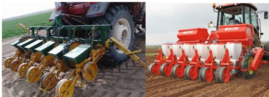
Fig. 11.16 Mechanical and pneumatic precision sowing machines used in sugar beet cultivation
