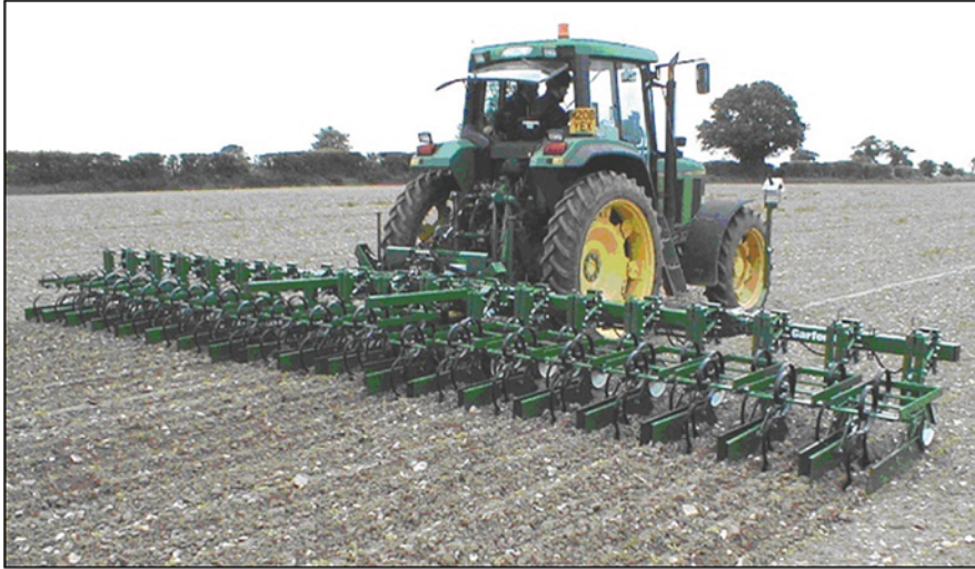
Fig. 17.5 Inter-row hoeing using crop protectors. Source: Cloutier et al. (2007)
