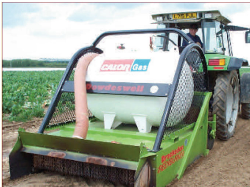
Fig. 17.14 Infrared weeder. Source: Merfeld (2011)
