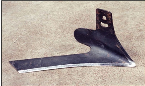
Fig. 17.17 An L sweep blade. Source: DEFRA (2002)
