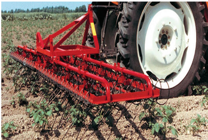
Fig. 17.10 Spring or flexi tines. Source: Zeng et al. (2020)
