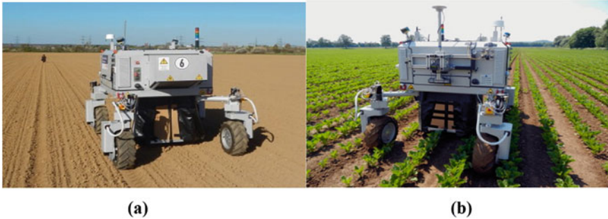
Fig. 17.25 Field robot BoniRob operating on the field. (a) Data acquisition 3 days after planting, (b) data acquisition 5 weeks after emergence. Source: Chebrolu et al. (2017)
