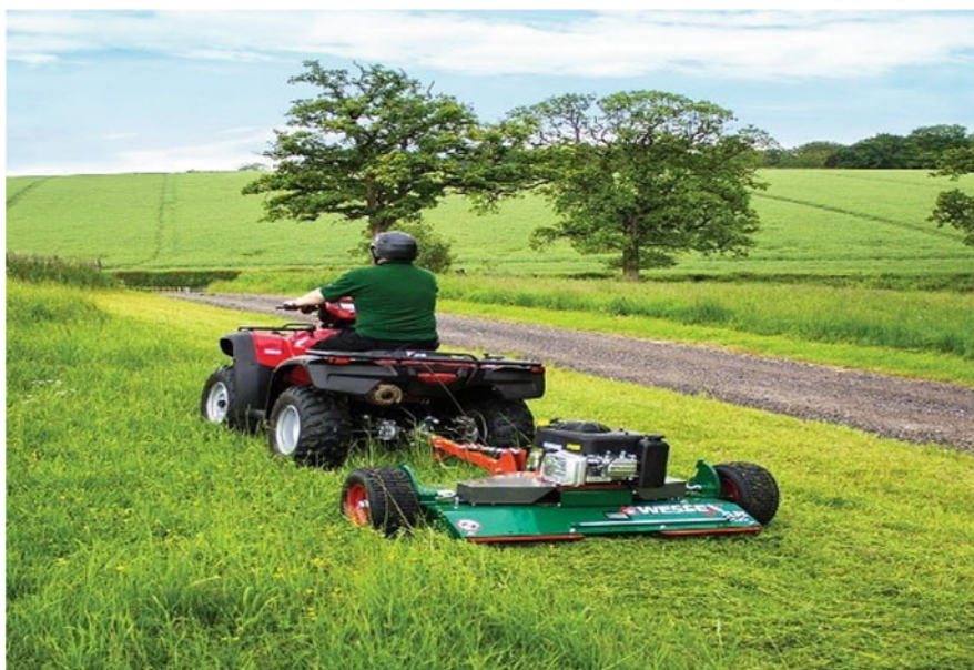
Fig. 17.12 Mower or topper. Source: Pathade et al. (2015)
