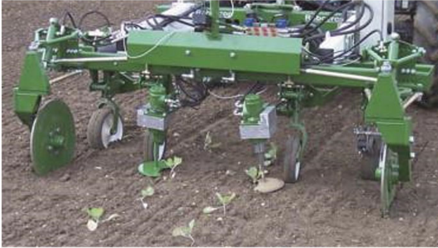
Fig. 17.20 A weeder with computer vision. Source: Tillett et al. (2008)
