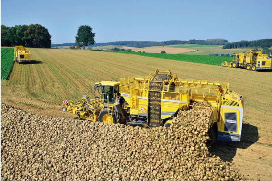
Fig. 24.24 Beet harvesting machine
