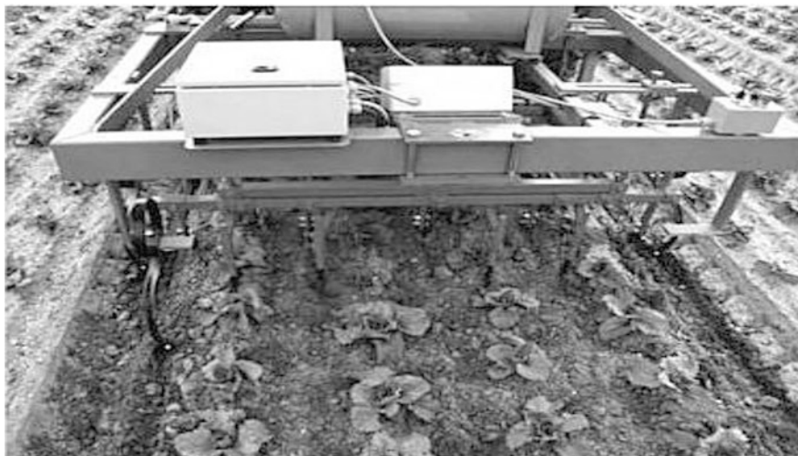
Fig. 17.21 An automated hoe weeder. Source: Cloutier et al. (2007)
