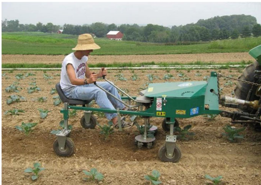
Fig. 17.9 ECO weeder. Source: HCC (2011)
