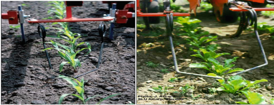
Fig. 17.7 Torsion weeder. Cloutier et al. (2007)
