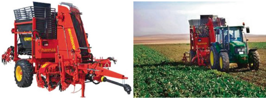
Fig. 24.31 One-row trailed harvester
