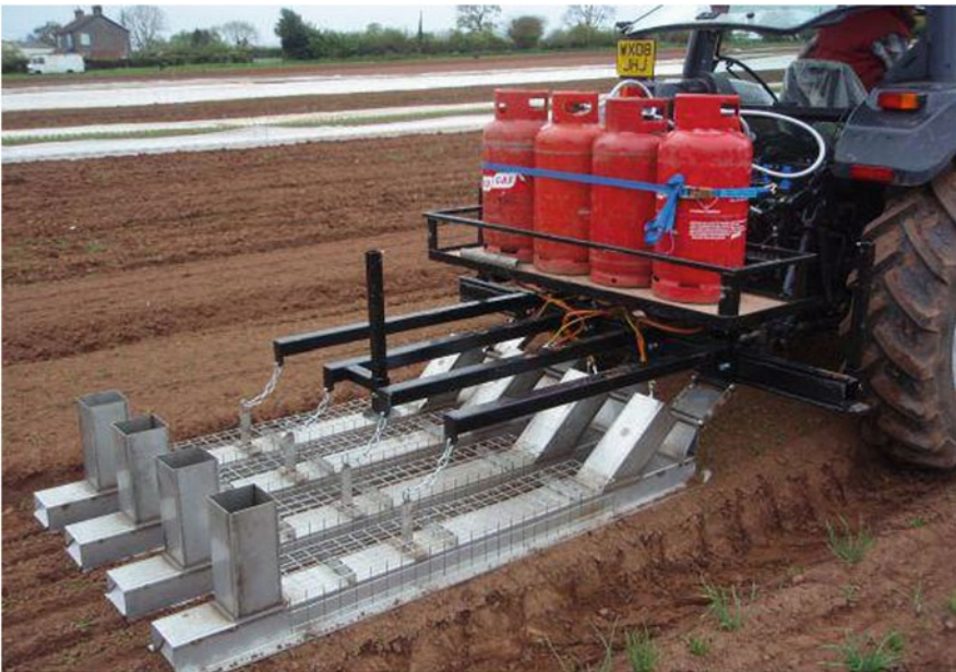
Fig. 17.13 Flame weeder. Source: Merfeild (2011)
