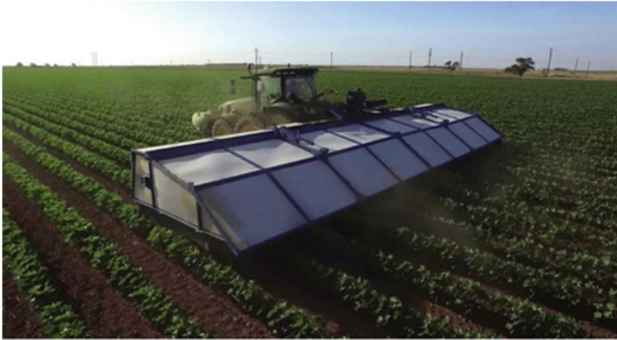
Fig. 17.27 The See & Spray robot. Source: Blue River Technology (2018)
