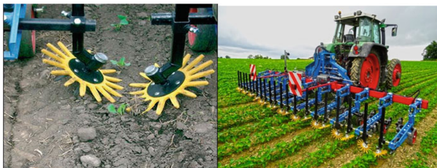
Fig. 17.6 Finger weeder. Cloutier et al. (2007)
