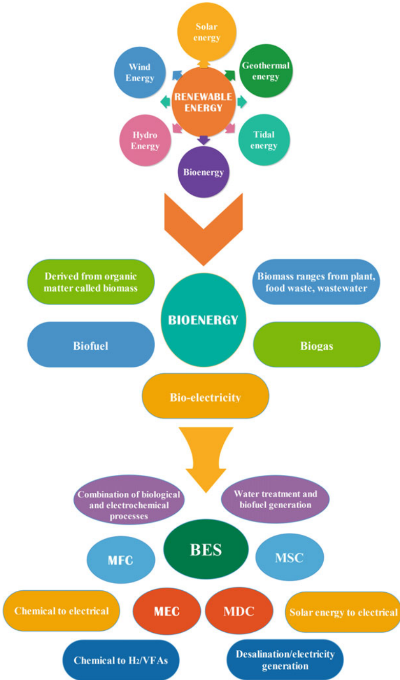
Fig. 5 Flow diagram showing different sources of renewable energy with special reference to bioenergy
