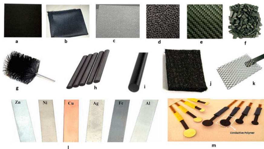
Fig. 1 List of commonly used electrodes: a carbon paper, b carbon cloth, c carbon fiber, d reticulated vitrified carbon, e carbon mesh, f graphitic granular, g carbon brushes, h graphite rod, i polycrystalline graphite, j carbon felt, k platinum mesh, l different metal electrode strips, and m conductive polymer-based strips. Adapted from reference [25] with MDPI permission
