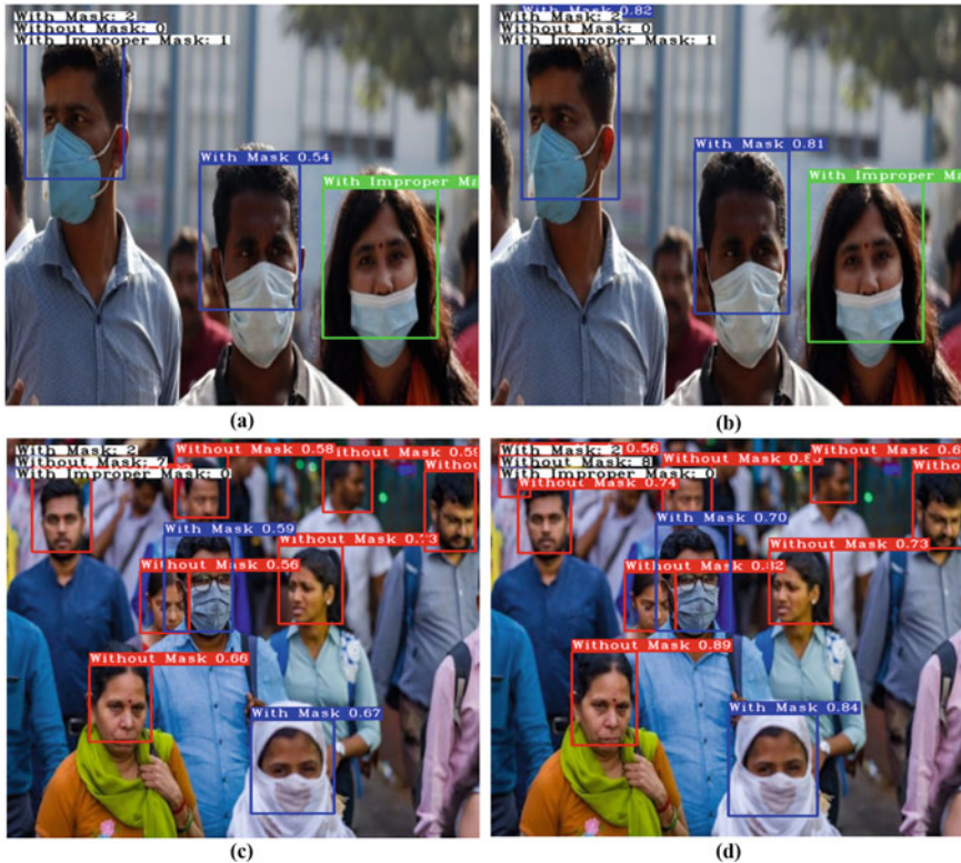
Fig. 5 Real-time testing results: a and c from YOLOv3 Tiny, and b and d from YOLOv4 Tiny
