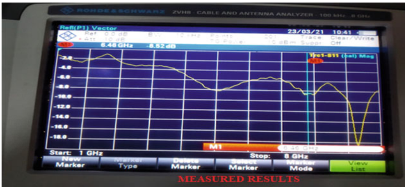
Fig. 10 Measured return loss of the prototype
