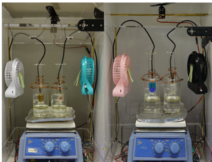
Fig. 8.2 Photo of two sets of OEs for investigating exothermic crystallization of sodium acetate from its supersaturated solution
