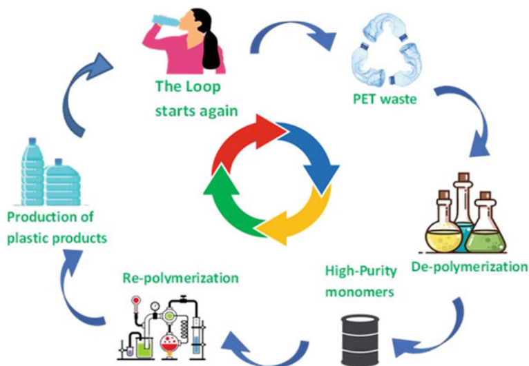
Fig. 3 Schematic representation of the steps involved in chemical recycling of PET waste
