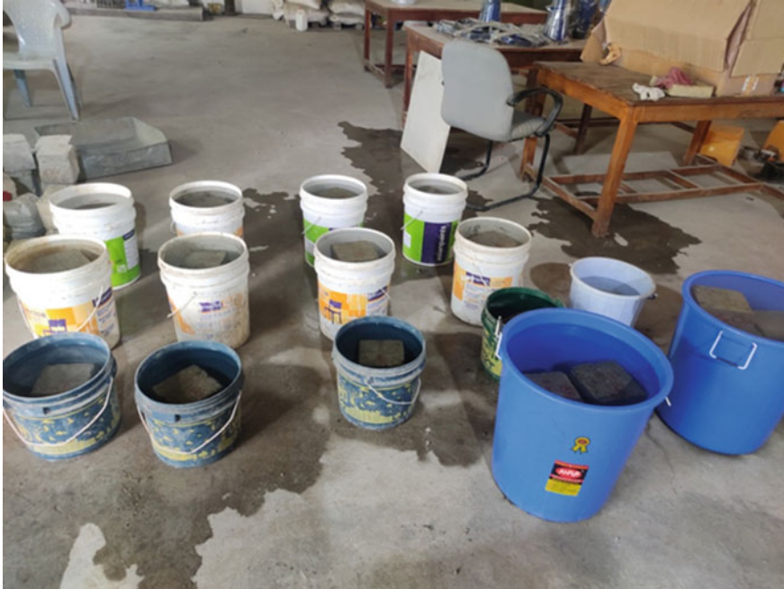
Fig. 1 Representing the curing of concrete blocks
