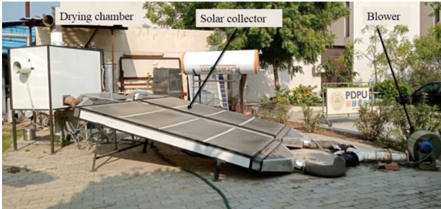
Fig. 4 Forced convection solar dryer
