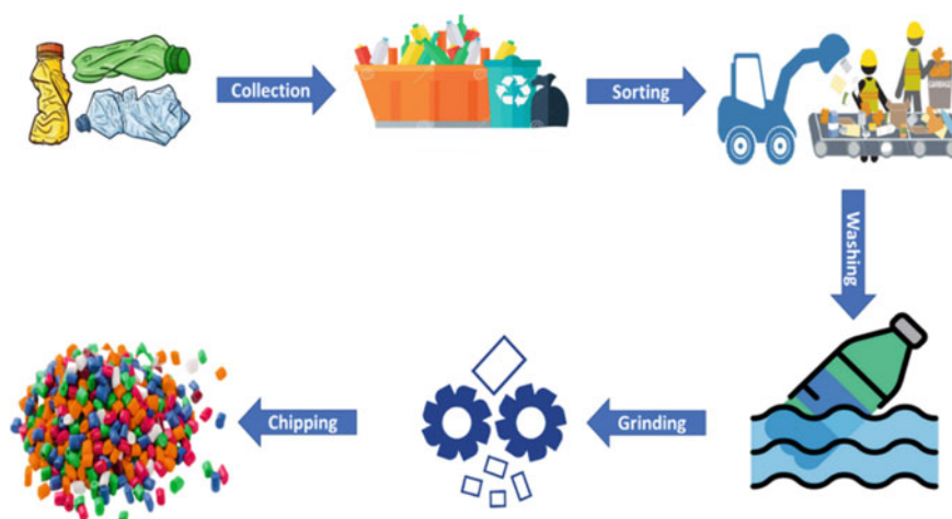
Fig. 2 Schematic representation of the steps involved in mechanical recycling of PET waste
