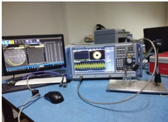
Fig. 2 DAK liquid dielectric assessment system showing measurement on DAK software using DAK 3.5 probe and ZNB 8 VNA
