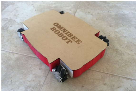
Fig. 9 OMNIBEE omnidirectional mobile robot
