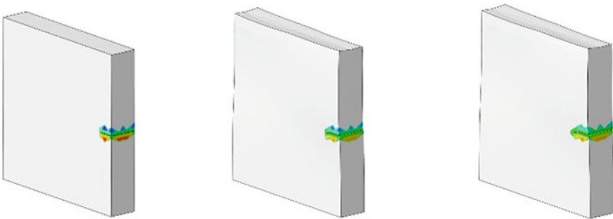
Fig. 17 Progressive crack growth in lamina due to 0-400-0 MPa load up to 1000 cycles
