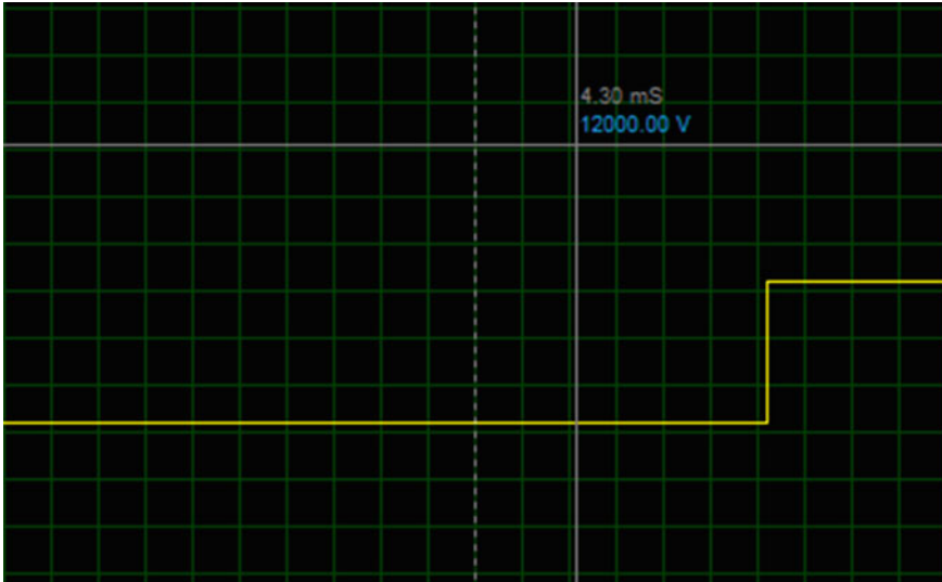
Fig. 15 Simulation of the output of high-voltage spark (12 kV)
