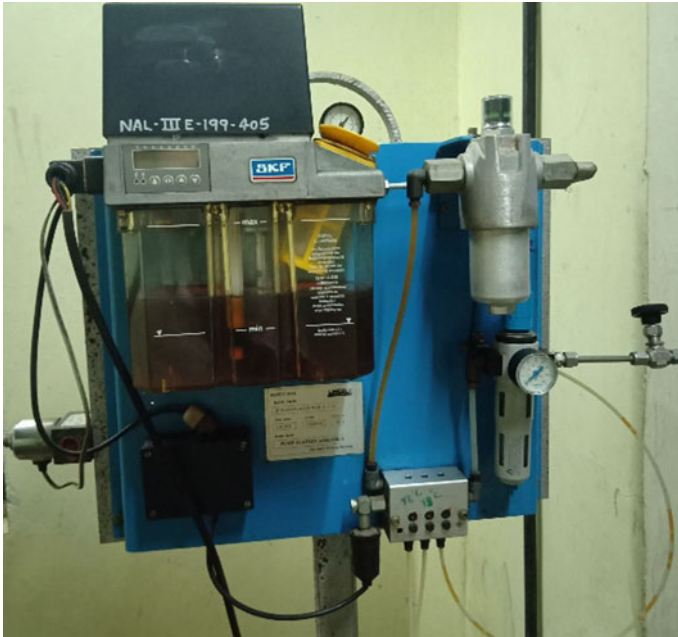
Fig. 7 Oil air mixture generator
