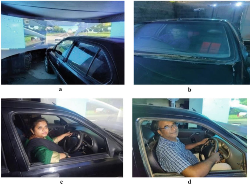
Fig. 10 Driving simulator setup and testing a Driving simulator setup (Front view with screen). b Driving simulator setup (Back view with projectors). c Female subject participation. d Male subject Participation
