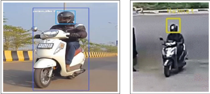
Fig. 1 Sample result obtained with YOLOv4 model for the task of helmet detection
