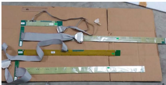
Fig. 143.3 Hall probe PCBs
