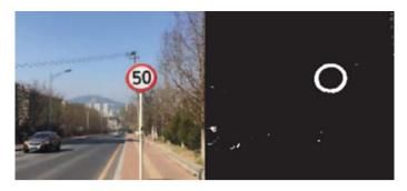
Fig. 5 Segmentation of the HSV color space
