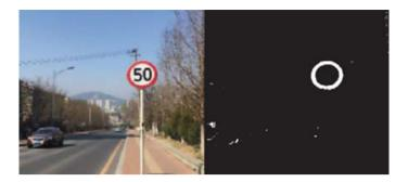
Fig. 4 Color space detection using RGB and HSV
