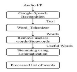
Fig. 2 Audio to processed text dataflow
