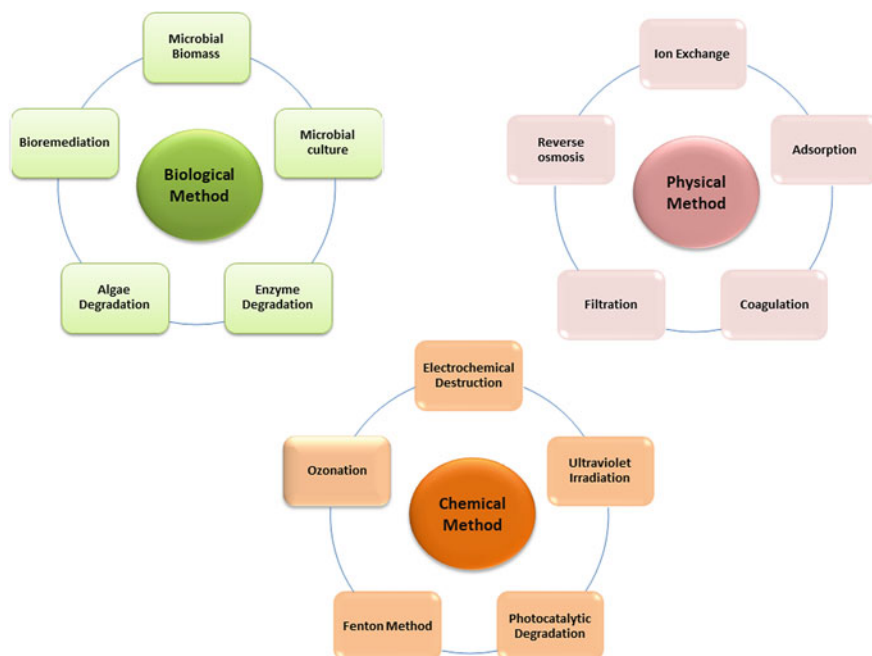
Fig. 5 Schematic illustration of biological, physical and chemical dye removal method
