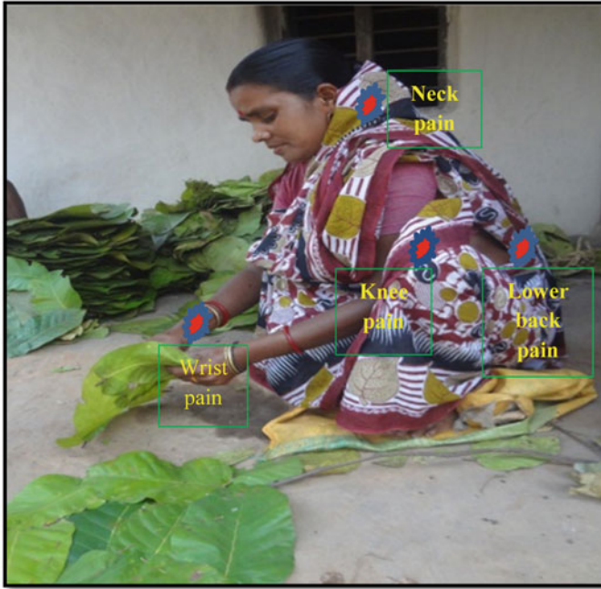
Fig. 5 The posture maintained by the female workers during stitching of Sal leaves the plate
