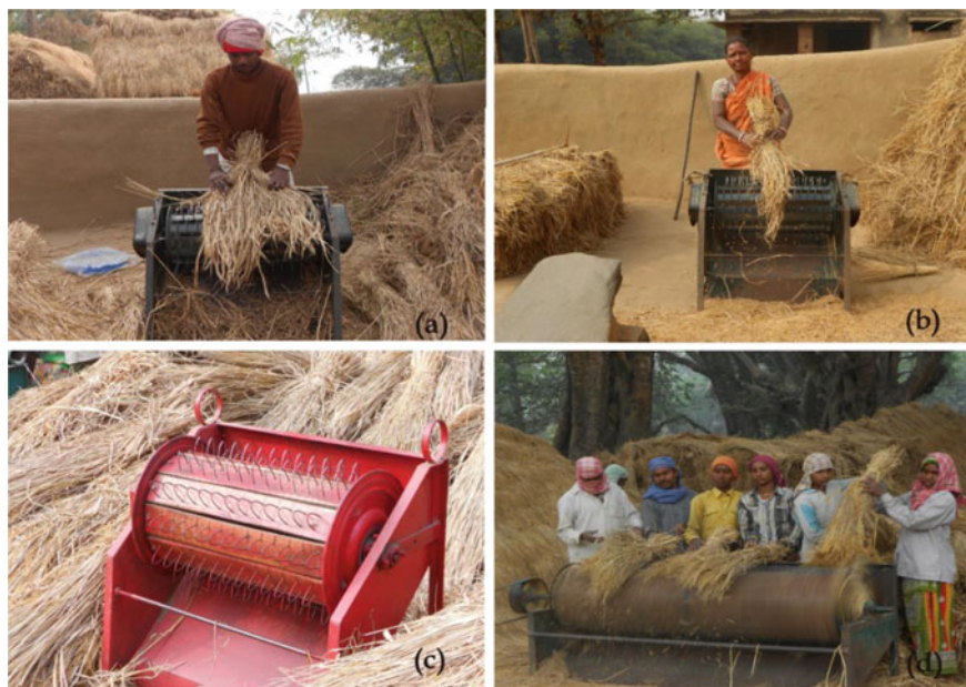
Fig. 1 a, b Workers engaged in threshing paddy with pedal thresher; c pedal thresher; d workers engaged in paddy threshing with power thresher
