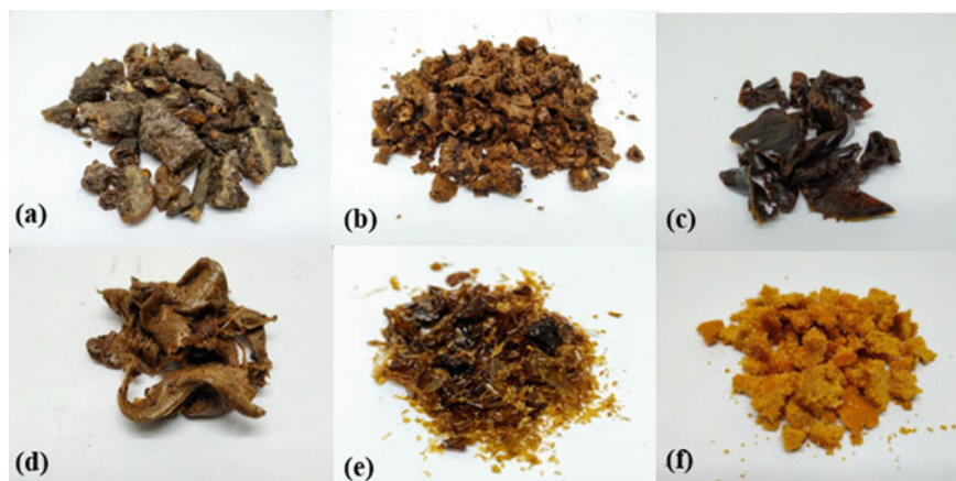
Fig. 6 a Crude lac, b collected lac resin post first wash, c extruded lac resin dissolved in IPA, dried, d collected lac resin post third wash, e final lac resin product post washing and extrusion, and f commercial button lac dissolved in IPA and dried
