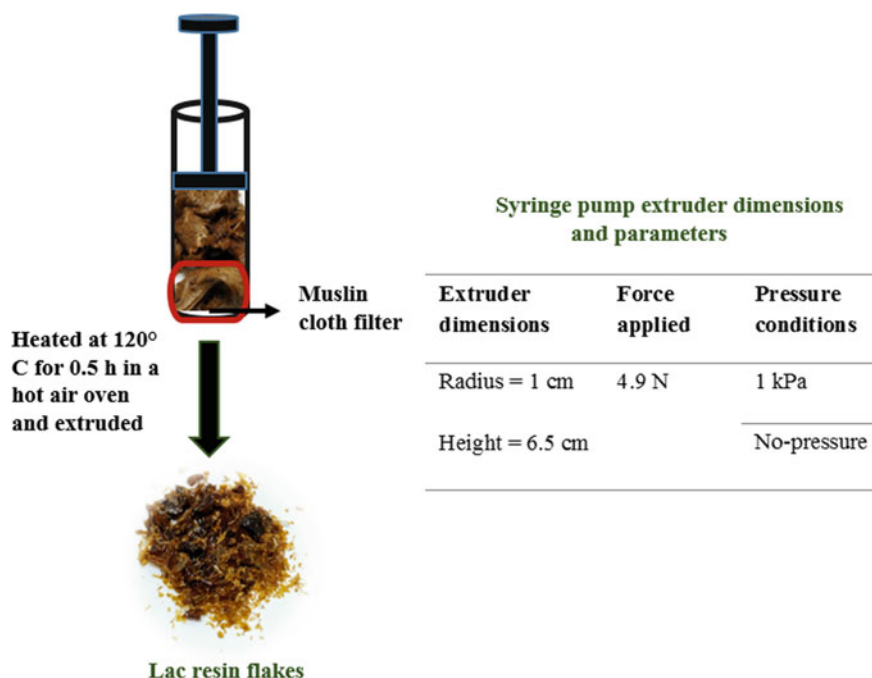
Fig. 2 Schematic diagram representing the syringe pump hot extrusion setup and extrusion parameters
