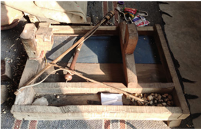
Fig. 2 Traditional hand-operated lathe like device for making Tulsi beads
