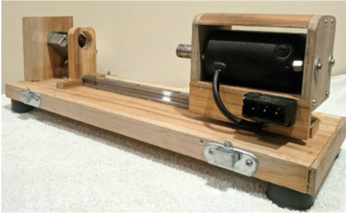
Fig. 7 New Tulsi beads making device of RuTAG IIT Delhi powered by AC motor
