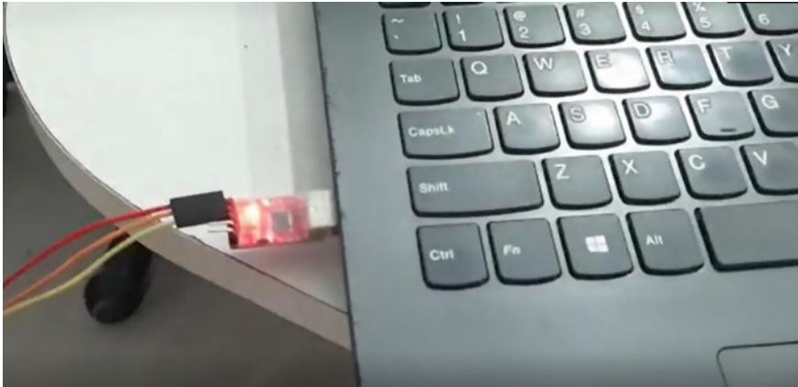
Fig. 5 LoRa receiver connected to the USB port of the computer to receive the GPS co-ordinates
