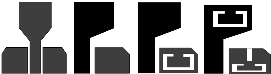
Fig. 2 Design development of the ACS Monopole antenna
