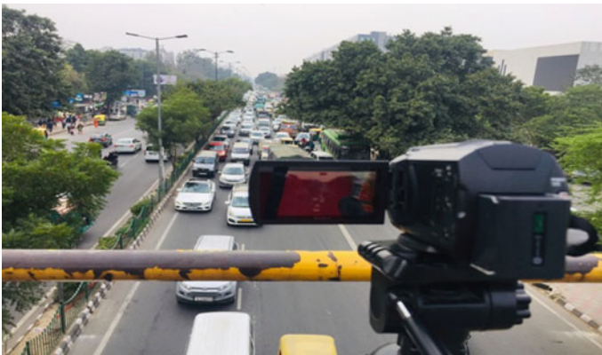
Fig. 5 Handycam setup at foot over bridge for data collection
