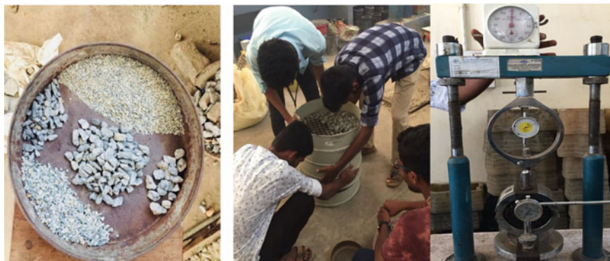
Fig. 1 Sieving and collection of aggregates, Marshall stability testing of SMA mix
