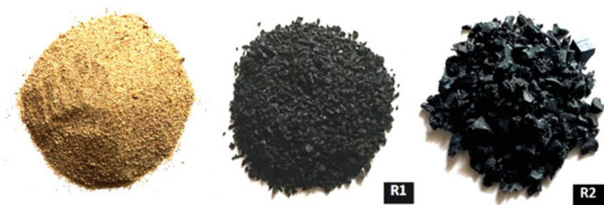
Fig. 1 Sand and rubber samples, R1 and R2 used in the present study
