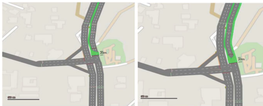
Fig. 5 Modified model with two-wheeler box a case 1 and b case 2. The box length, from STOP line, considered in this test cases is 20 m as indicated
