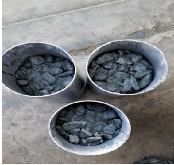
Fig. 2 Casting pervious concrete in PVC pipes
