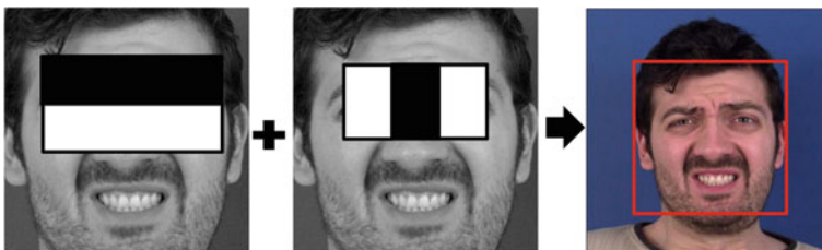
Fig. 2 Face detection using Haar Cascade Classifier
