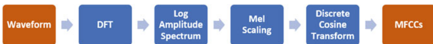
Fig. 1 Process of obtaining MFCCs. This figure explains all the steps needed to obtain the MFCCs of a given waveform
