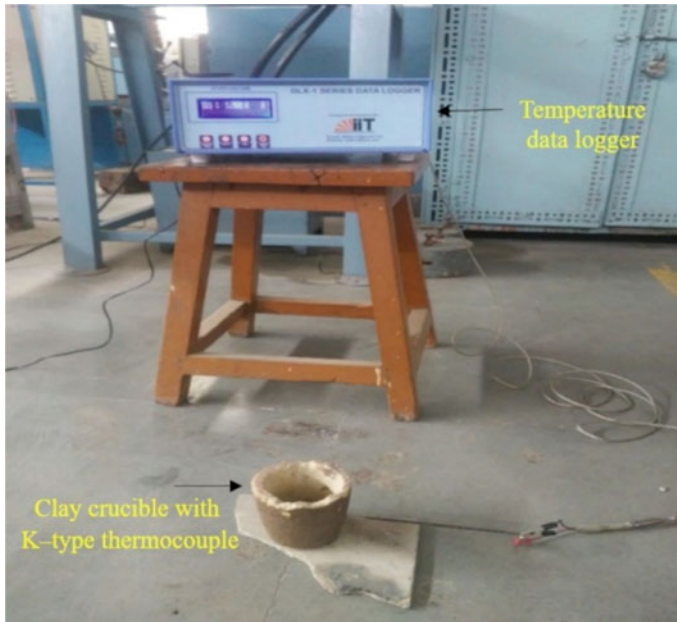
Fig. 9.1 Experimental set-up for cooling curve analysis
