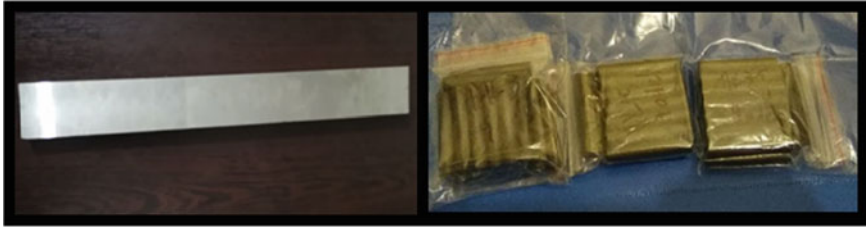
Fig. 75.4 Grinded workpiece and cylindrical graphite bars HK3-HK15-HK75 [14]
