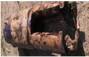
Sandblasting mouth of conventional sand jet broken after adding 80m 3 sand
