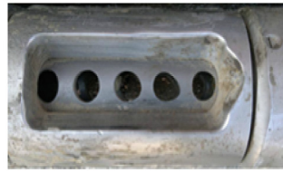
Sandblasting mouth after optimization slightly corroded when adding 516m 3 sand injection design
