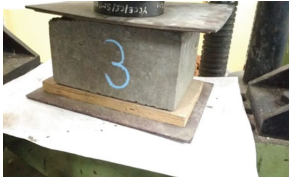
Fig. 11 Compressive strength test on third sample of the brick
