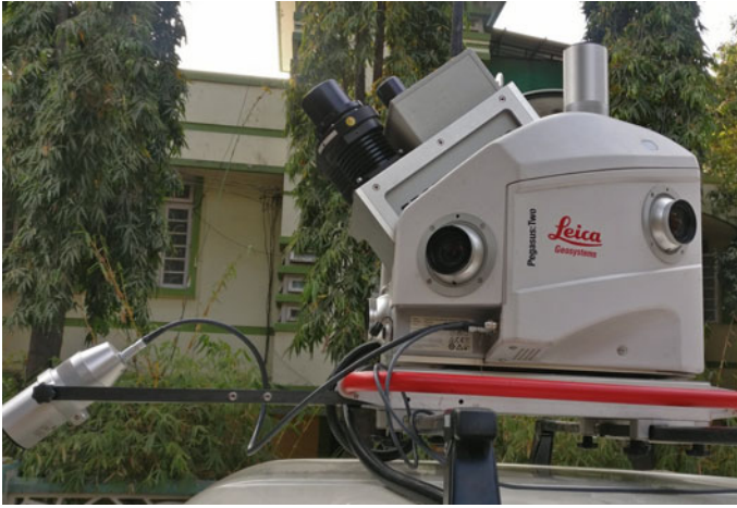
Fig. 1 Data capture on site by mobile LiDAR, “Leica Pegasus Two” for 2.8 km road in Pune
