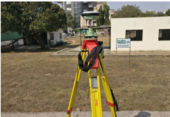
Fig. 6 Leica GS14 dual frequency DGPS receiver kept as a base station on ground for GPS observations in static mode
