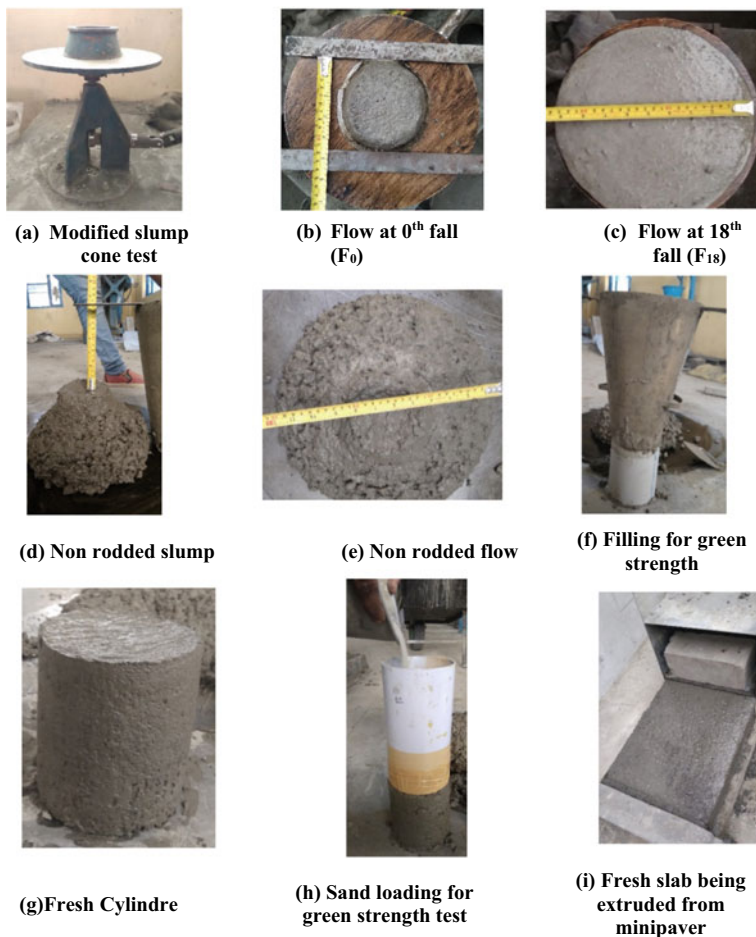
Fig. 6 Steps involved in laboratory production of the SFSCC
