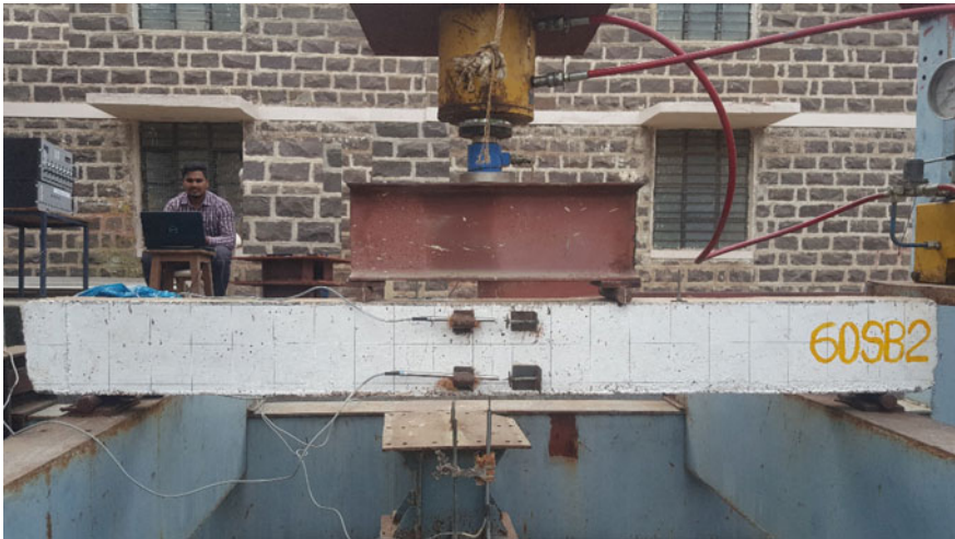
Fig. 3 Experimental setup for HPC beam 60SB2
