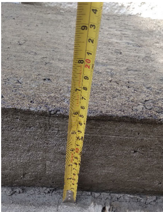
Fig. 7 Shape stability and surface quality of the fresh SFSCC slab extruded from the minipaver system
