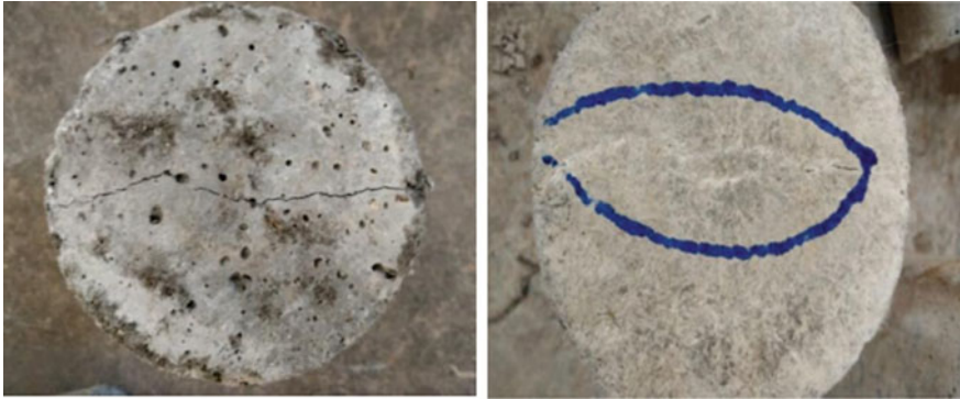
Fig. 8 Healing of concrete cylinder due to microcapsule
