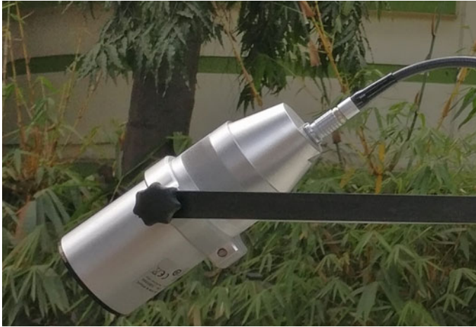
Fig. 2 Enlarged view of the pavement camera attached to the mobile LiDAR, “Leica Pegasus Two”
