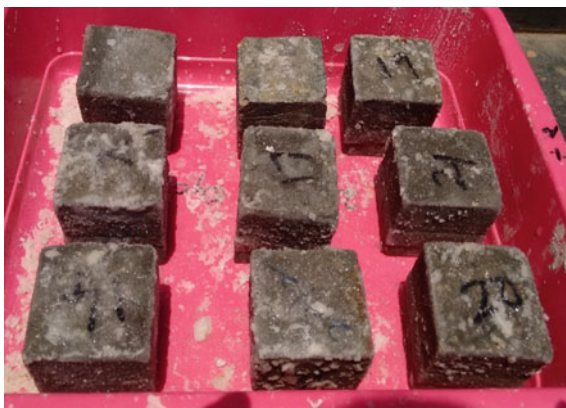
Fig. 6 Salt crystals in FRPC samples
