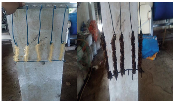
Fig. 2 Ring lace media used before the growth of biomass and after the growth of biomass
