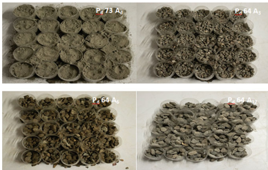
Fig. 3 A view of the plastic bottle mattress “ P_d 73 ” with cellular pocket infill with 3, 6, 12 in mm and quarry dust aggregate grading
