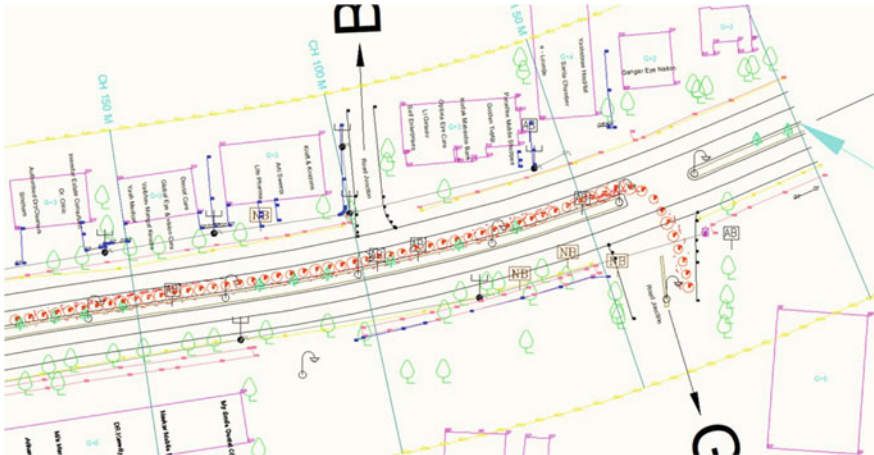
Fig. 4 Screen shot of the “Crack Index” in red circles, with the topographic features of the road
