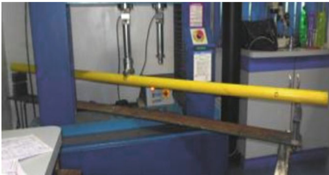
Fig. 2 3-point load testing of pultruded pipe
