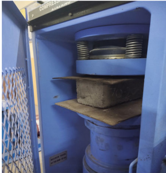
Fig. 7 Compression test on brick specimen
